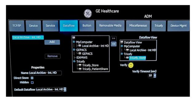
To configure the End Exam button to archive the entire study, move the Tricefy\_store into the Dataflow View. To configure the button to send the entire study to a patient, move the Tricefy\_Patientshare.
