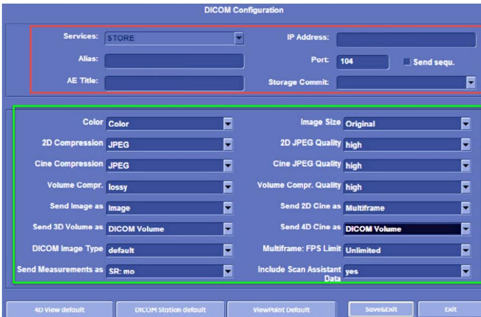
By default, the compression settings, shown above in the green box, will have to be adjusted. Don't worry, adjusting these settings will not lower image quality. Modify the compression settings to match the following:
