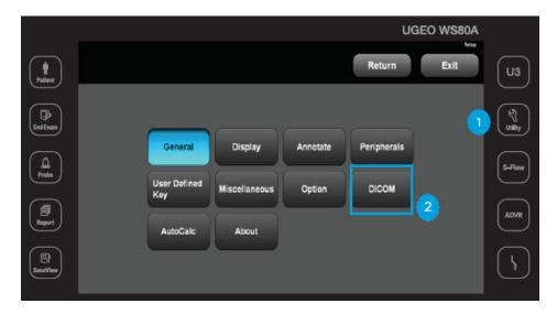
The DICOM Configuration screen will display. This screen allows you to add new DICOM stores. These stores are like warehouse receiving centers; they receive the data from your ultrasound system.
